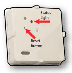
To clear the alarm, reset the system power, or press the reset button (using a paperclip or toothpick) which will automatically clear the alarm on the unit.
