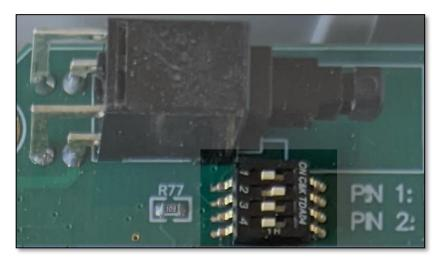
The Room Size switch setting enables the user to adjust the SA100 unit's detection sensitivity based on the physical room the unit is installed into.
